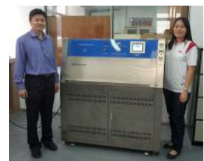
UV Accelerated Weathering Chamber at University of Malaya
